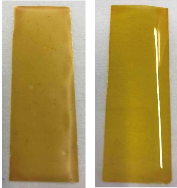
*Figure 17.* Two finished PI/SiO<sub>2</sub> samples, created through ex situ process (left), and in situ process (right).
