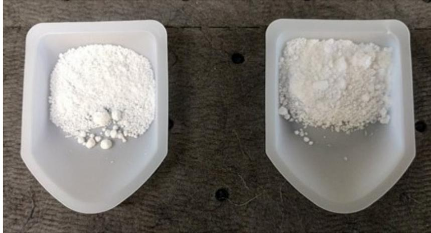
*Figure 9.* Silica particles purchased from Sigma-Aldrich, 20 nm (left) and 80 nm (right) in diameter.
